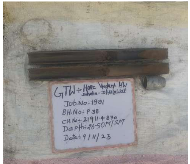
SPT sample at depth 26.50 m
