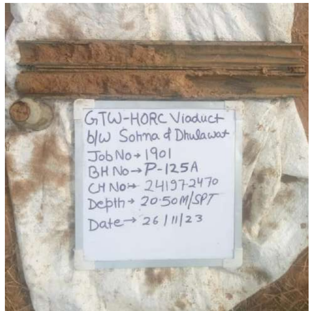
SPT sample at depth 20.50 m
