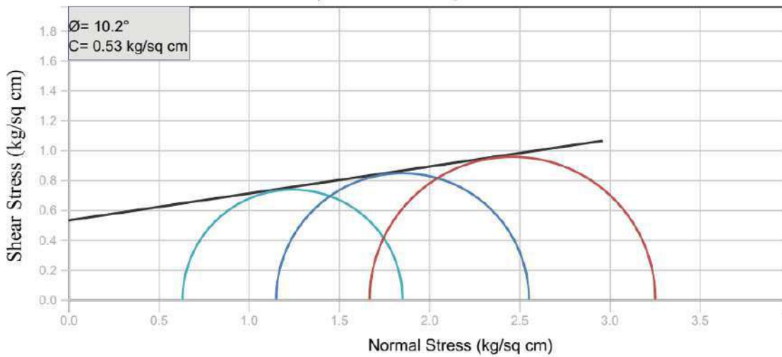
1901-HRIDC-VI-23588.287 BH-NO.P102, DEPTH-11.00M, TRIAXIAL GRAPH
