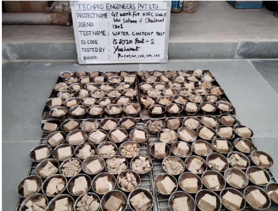
Water content test
