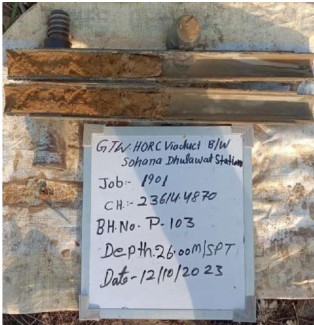
SPT sample at depth 26.00 m
