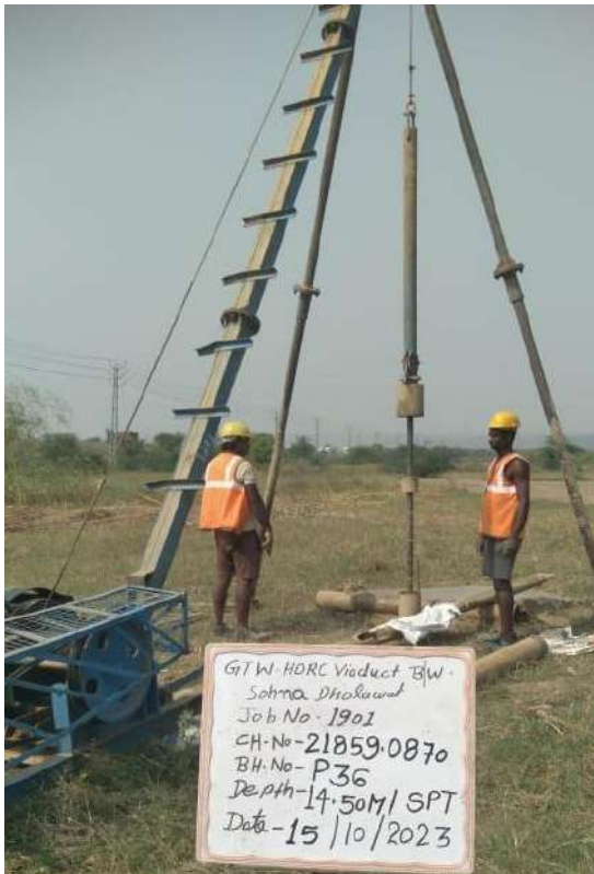
SPT at depth 14.50 m
