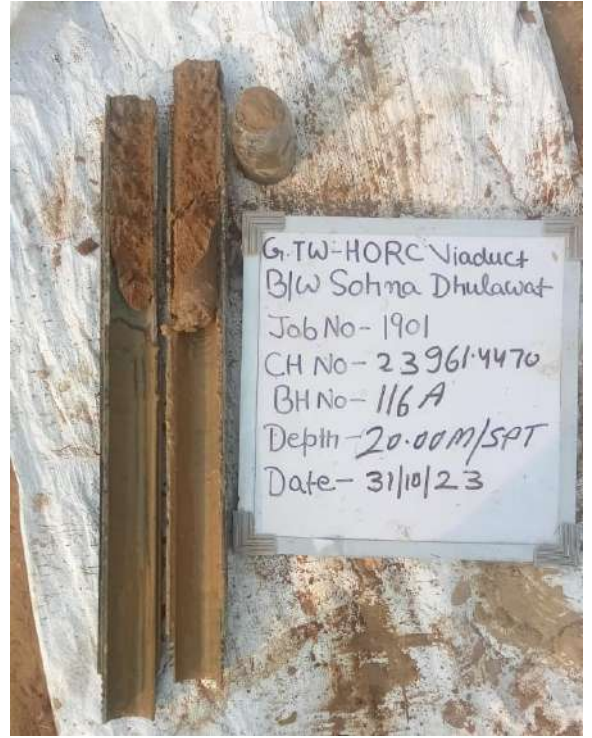
SPT sample at depth 20.00 m
