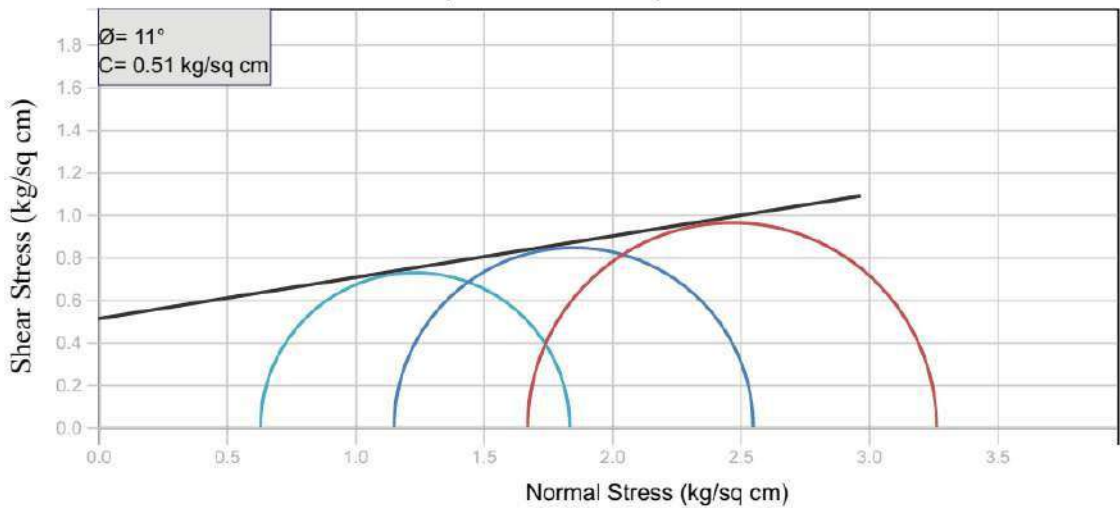
1901-HRIDC-VI-23640.687 BH-NO.P104, DEPTH-7.00M, TRIAXIAL GRAPH
