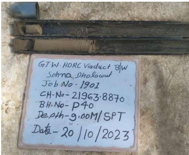
SPT sample at depth 9.00 m
