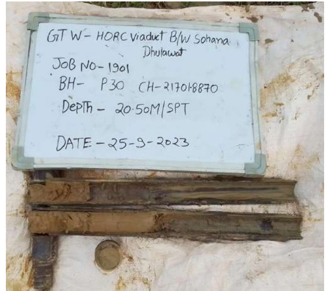
SPT sample at depth 20.50 m
