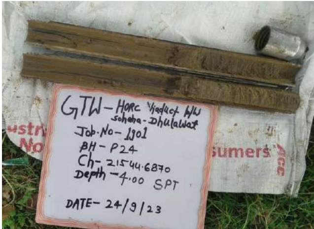
SPT sample at depth 4.00 m
