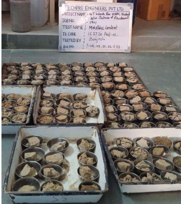
Water content test
