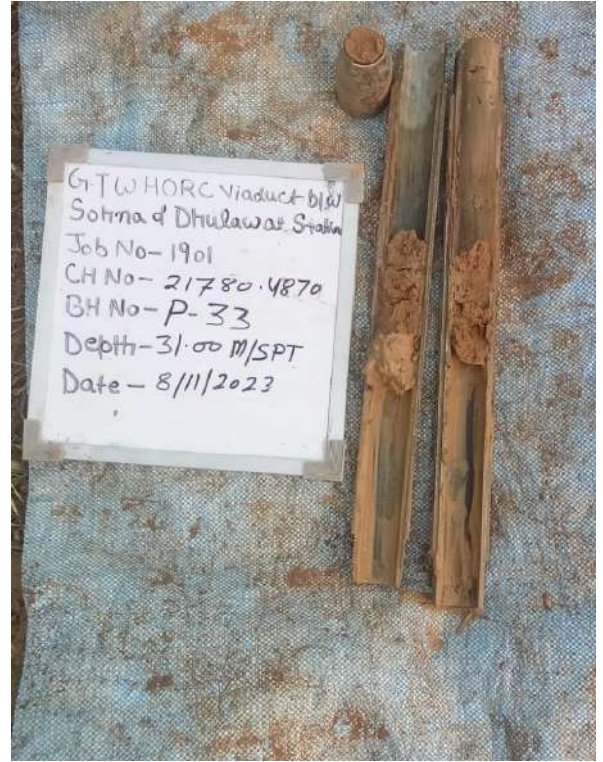
SPT sample at depth 31.00 m
