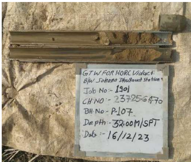
SPT sample at depth 32.00m
