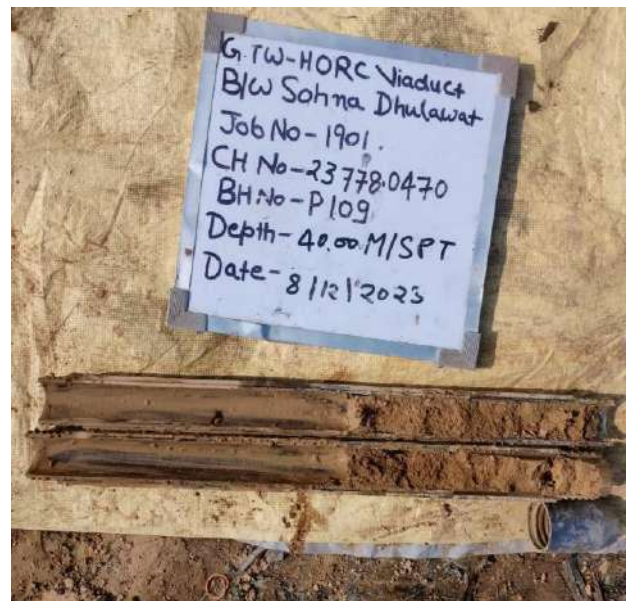
SPT sample at depth 40.00 m
