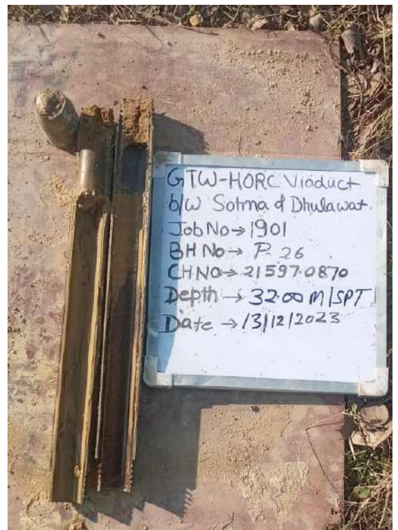
SPT sample at depth 32.00 m
