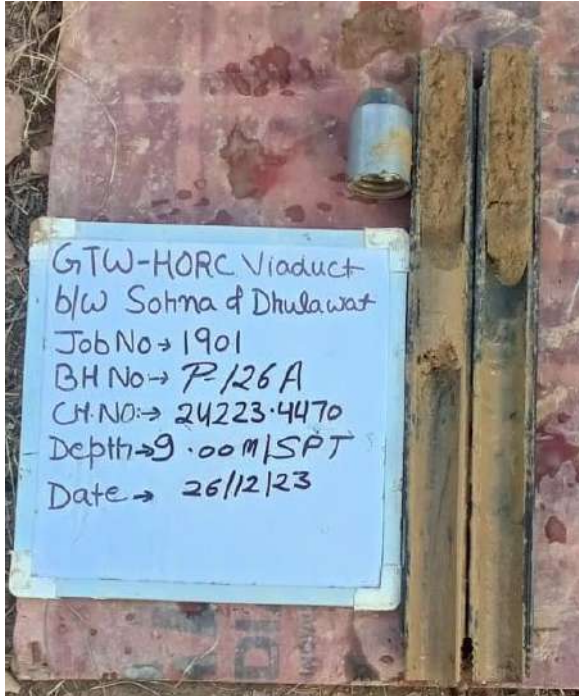
SPT sample at depth 9.00 m
