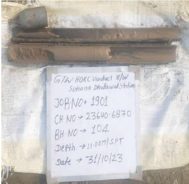
SPT sample at depth 11.00 m
