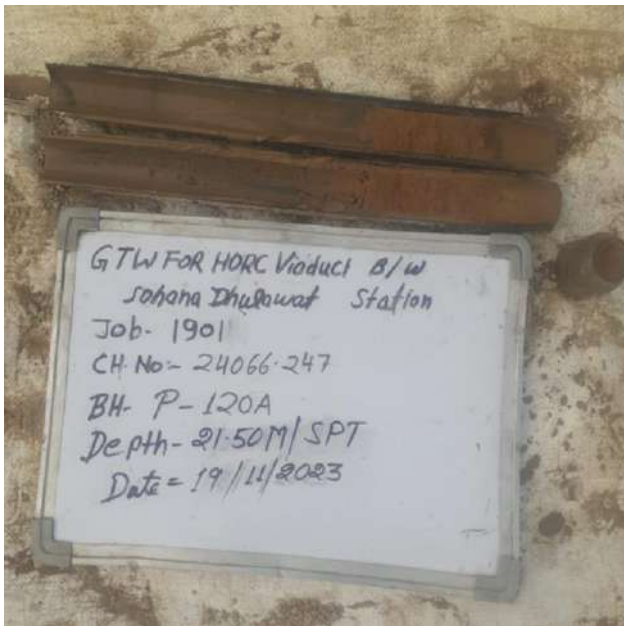
SPT sample at depth 21.50 m
