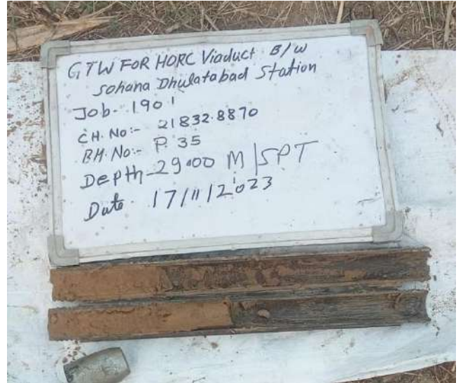
SPT sample at depth 29.00 m
