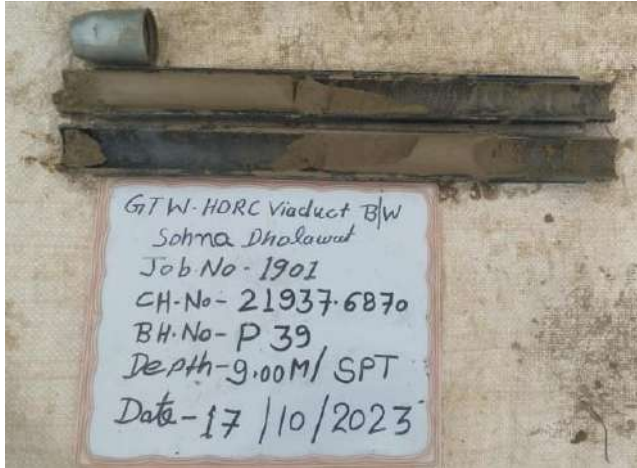
SPT sample at depth 9.00 m
