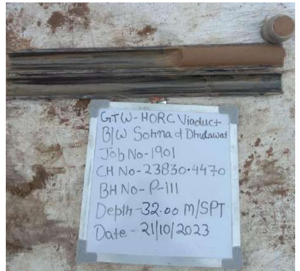
SPT sample at depth 32.00 m
